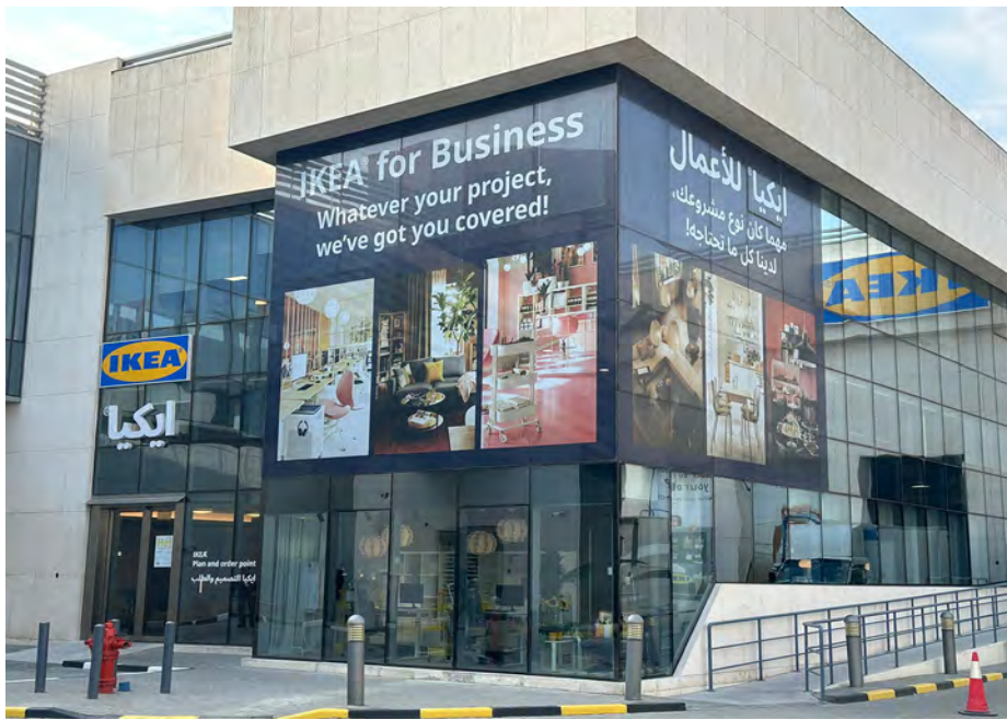
Form letter face lit sign made of acrylic and aluminum backing mounted with LED
